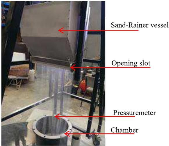
Figure 3. The automatic hopper to rain the sand into pressuremeter chamber test
