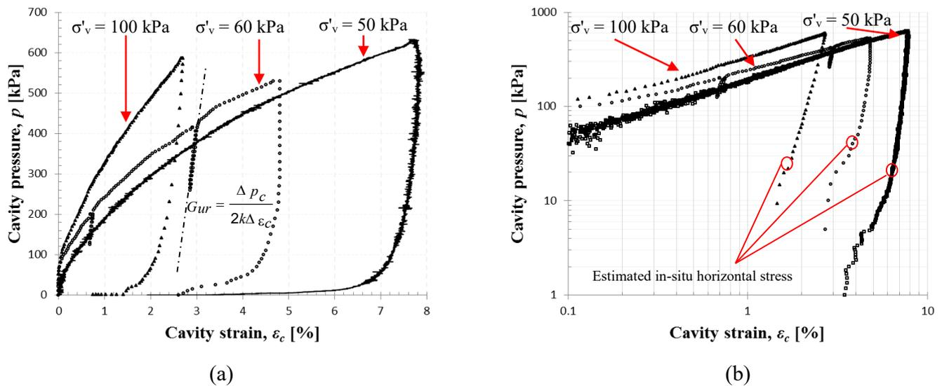
Figure 5. Measured variation of cavity pressure with cavity strain (a) linear scale and (b) logarithmic axes
