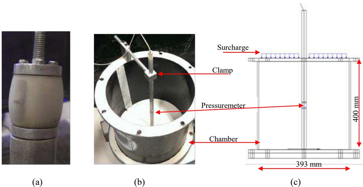
Figure 2. (a) Pressuremeter membrane, (b) pressuremeter in position prior to pouring sand (c) schematic diagram of the experimental set-up.
