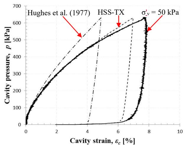
Figure 8. Comparison of measured pressuremeter response at  $\sigma'_v = 50$  kPa with HSS predictions using triaxial (TX) friction angles and friction angles calculated using Hughes et al. (1977)
