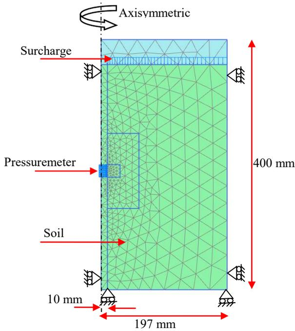
Figure 6. FE model of the experimental pressuremeter test.
