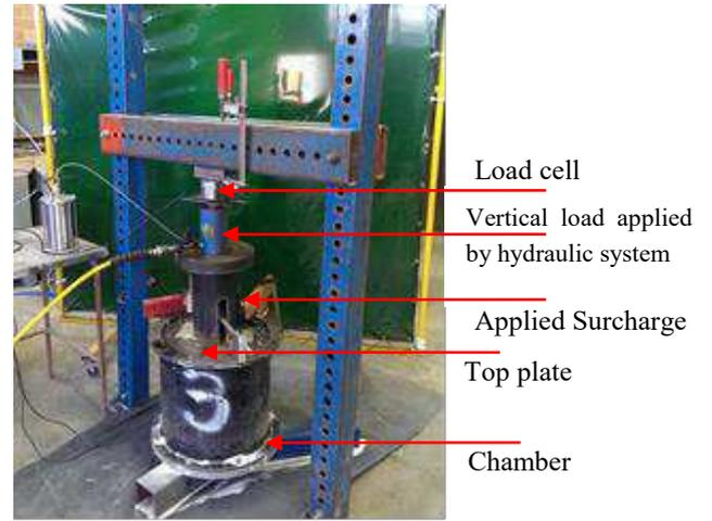
Figure 4. A typical pressuremeter test setup using a hydraulic system to apply the surcharge load
