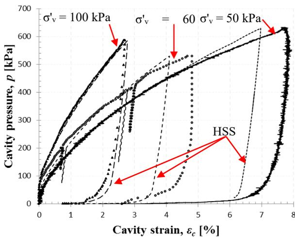
Figure 7. Hardening Soil-Small model for pressuremeter tests.
