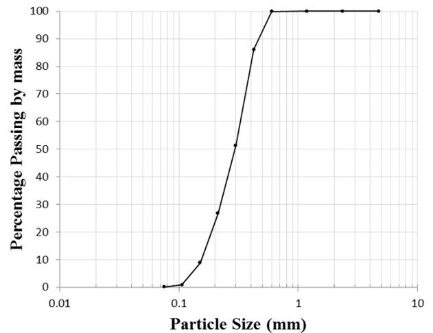
Figure 1. Particle size distribution of UWA fine silica sand
