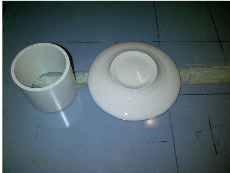
Figure 4 Photograph of a slump test with a miniature cylindrical mould.
