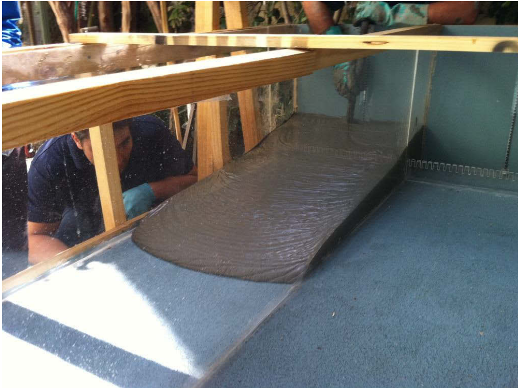
Figure 7 A laboratory flume test with glass sidewalls on thickened tailings. The photo is provided by Paterson & Cooke Chile.
