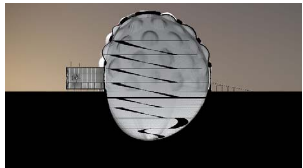
Figure 19: Section of exoskeletal geodesic structure with pressurized internal membrane project, Zachary Taylor, 2018.
