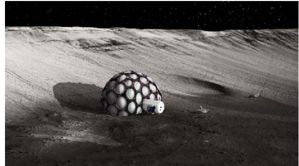
Figure 18: Perspective of exoskeletal geodesic structure with pressurized internal membrane project, Zachary Taylor, 2018.
