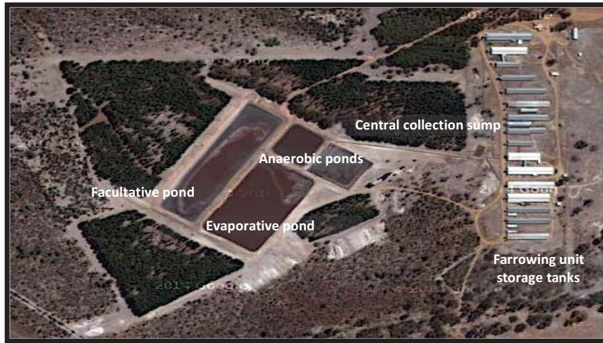
Figure 4.2 Onsite effluent treatment system at the piggery under investigation. Sampling points are marked
