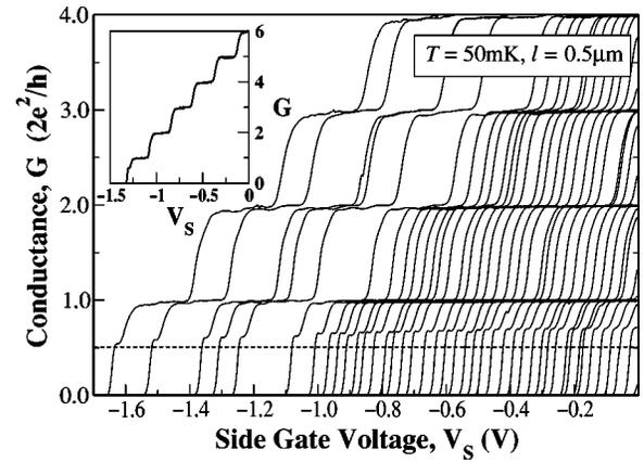
FIG. 2. Conductance of a  $l=0.5 \mu\text{m}$  quantum wire as a function of side gate voltage for  $V_T=560$  mV–1500 mV (right to left). Inset: Conductance as a function of side gate voltage for  $V_T=1.5$  V.
