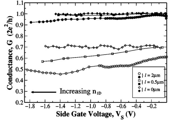
FIG. 4. Evolution of the conductance features (open symbols) seen in  $l=0, 0.5,$  and  $2 \mu\text{m}$  quantum wires as a function of  $V_S$ . The evolution of the corresponding  $n=1$  plateau near  $2e^2/h$  is also shown (solid symbols).
