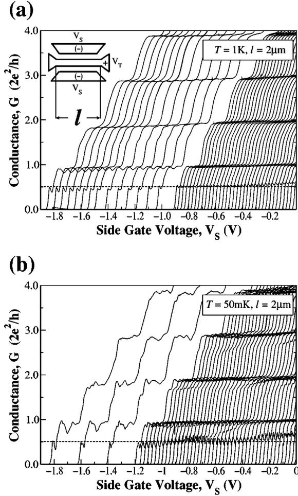
FIG. 3. Conductance of a  $l=2 \mu\text{m}$  quantum wire as a function of side gate voltage for  $V_T=300 \text{ mV}$ – $620 \text{ mV}$  (right to left). The data in (a) were obtained at 1 K and in (b) at 50 mK. The inset to (a) is a schematic of the device. Electrical conduction occurs below the middle region (top gate), which is biased positively with voltage  $V_T$ . The side gates are biased negatively with voltage  $V_S$ .  $l$  is the characteristic length of the 1D region.
