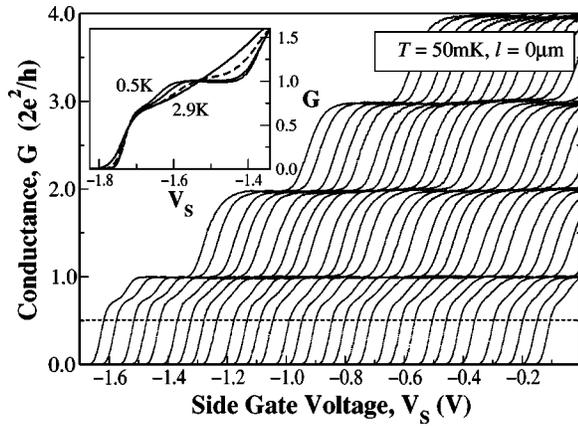
FIG. 1. Conductance of a  $l=0$  quantum wire as a function of side gate voltage for top gate voltages,  $V_T=172$  mV–300 mV (right to left) in steps of 4 mV. Inset: Temperature dependence of the conductance at  $V_T=0.4$  V for  $T=0.5, 1.0, 1.5,$  and  $2.9$  K.
