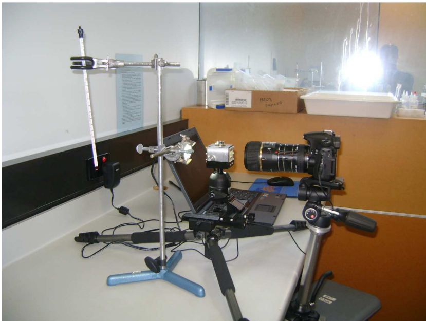
Figure 3.8 Modified captive drop IFT cell
