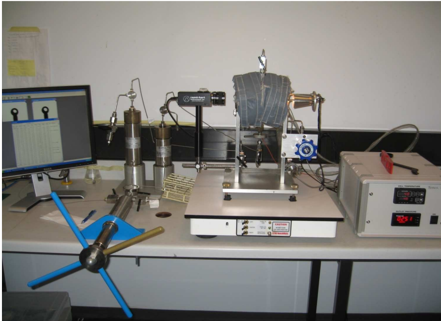
Figure 3.7 Temco pendant drop IFT cell
