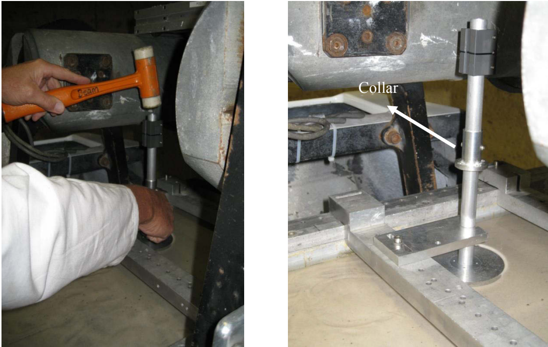
Figure 4-6. All piles were hammered to the required depth with a secured plate in place (after Harloe 2010)
