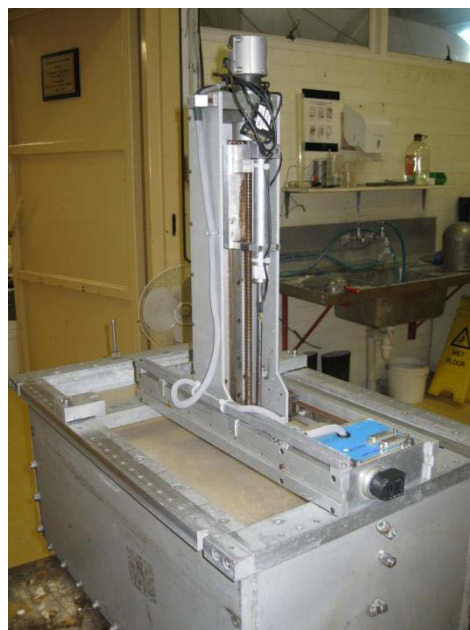
Figure 4-4. Motor driven actuator located on top of the strongbox (after Harloe 2010)
