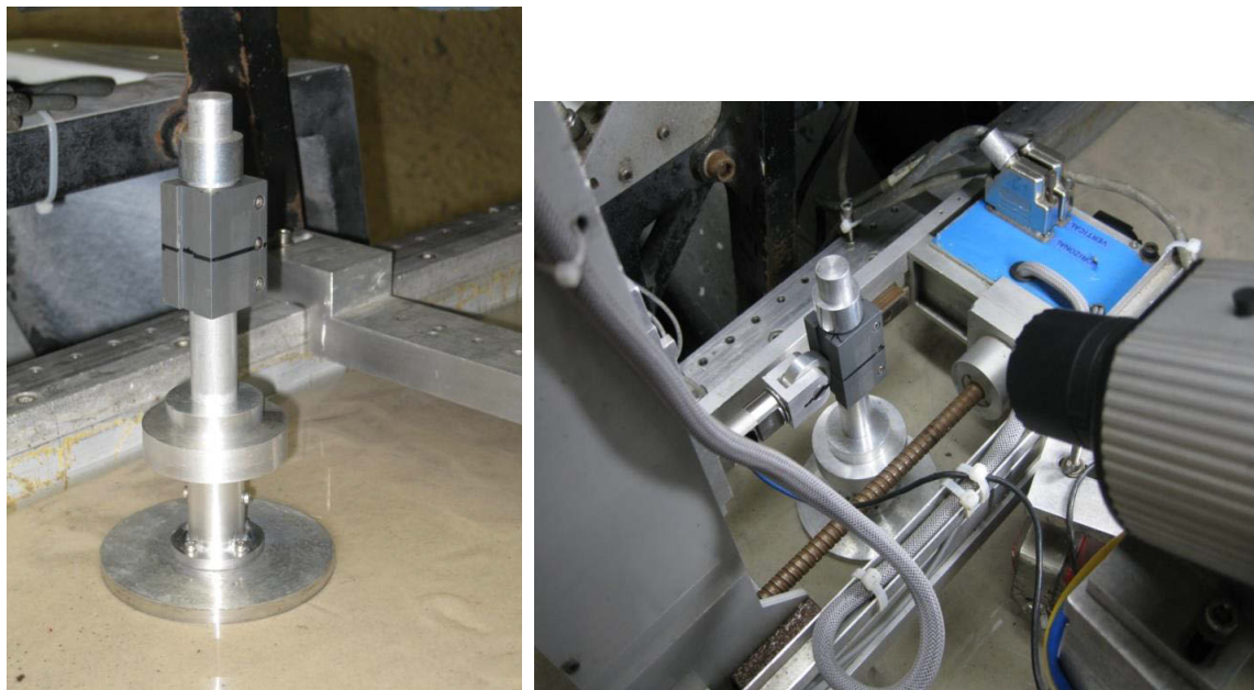
Figure 4-33. The piled footing structure installed in the silica sand (test number six) (after Harloe 2010)
