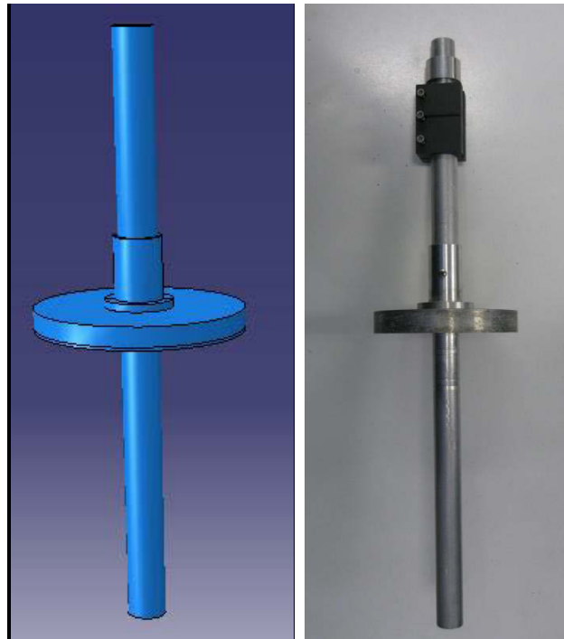
Figure 5-49. The piled footing structure constructed for model number three (piled footing, VL=6.5 MN)
