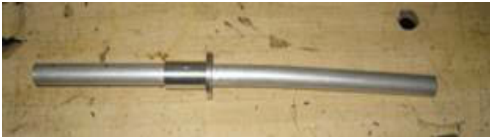
Figure 4-19. The yielded aluminium bar (test number one) (after Harloe 2010)
