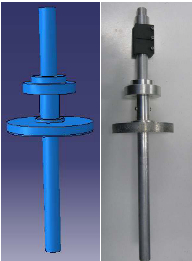
Figure 5-73. The assembled structure for model number five (piled footing)
