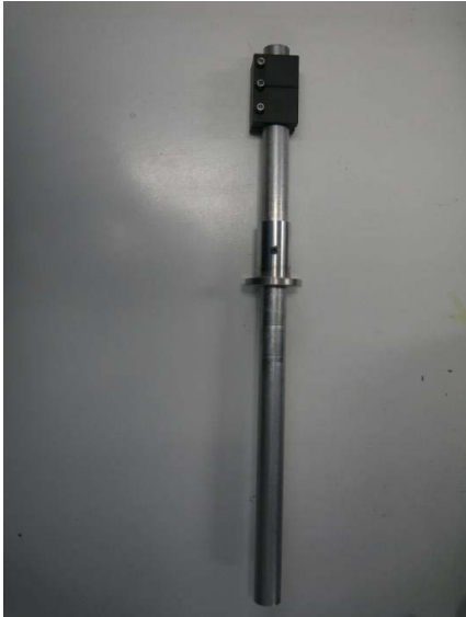
Figure 4-17. The hollow pipe with the collar and the load application piece (test number one) (after Harloe 2010)
