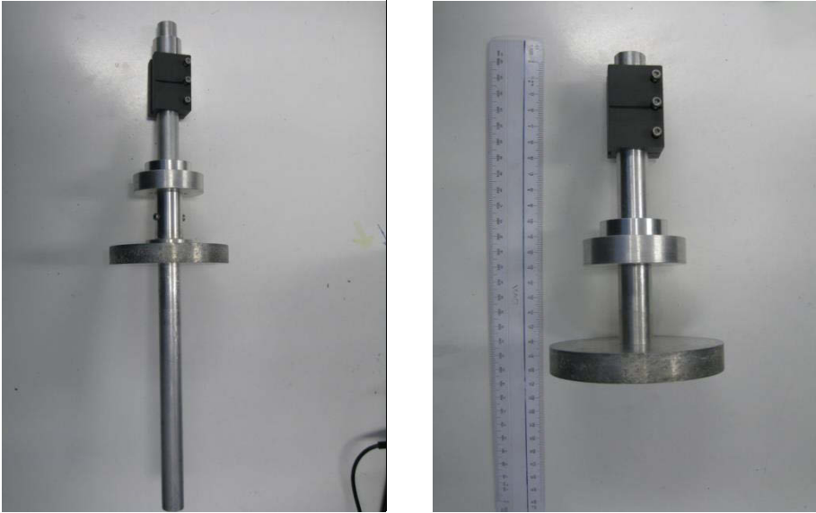
Figure 4-15. Footings number two and three were used to increase the vertical loads on the single footing and the hybrid structure during the tests (Table 4-4) (after Harloe 2010)
