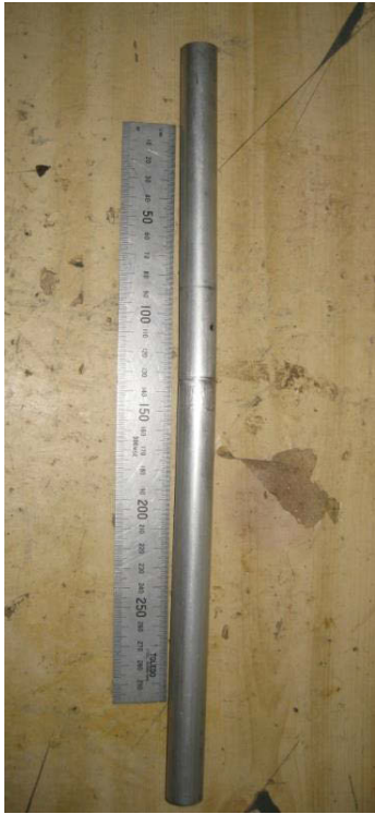
Figure 4-25. The yielded aluminium bar after test number three was completed (after Harloe 2010)
