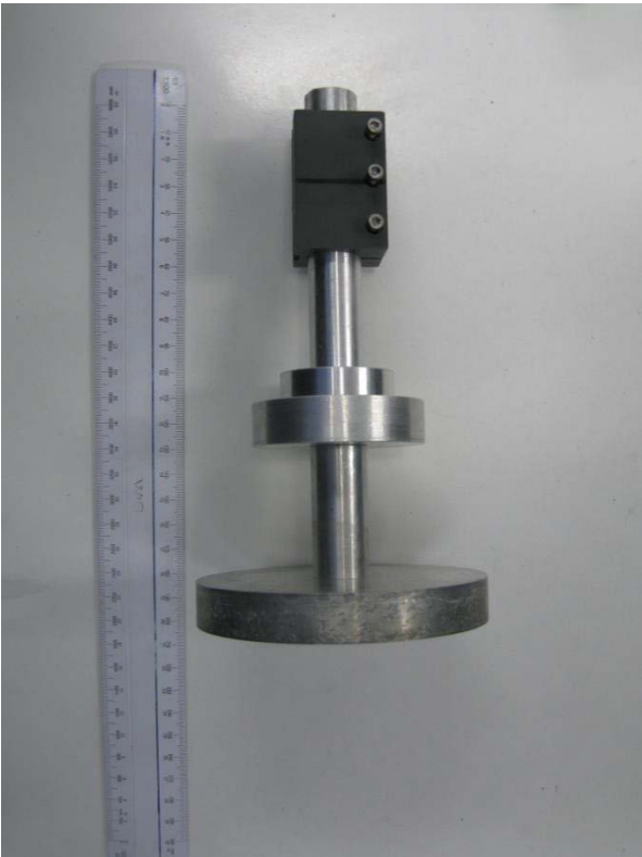
Figure 4-35. The single footing structure in test number seven (Single footing) (after Harloe 2010)
