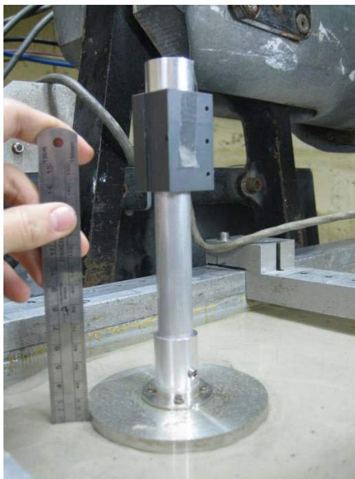
Figure 4-23. The location of the load application piece in test number three (Piled footing structure) (after Harloe 2010)
