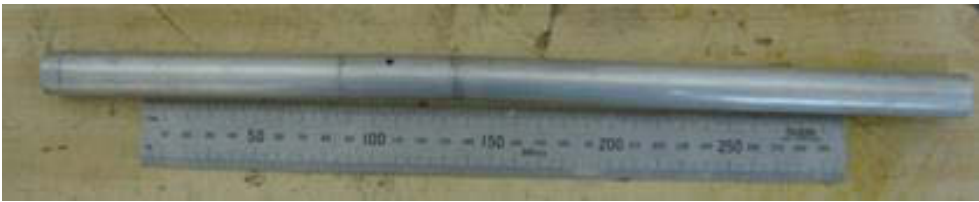
Figure 4-31. The yielded pile after test number five was completed (after Harloe 2010)
