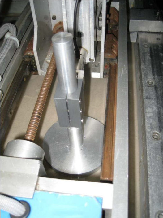
Figure 4-20. Test number two, the footing and the solid tower used during the testing programme (after Harloe 2010)
