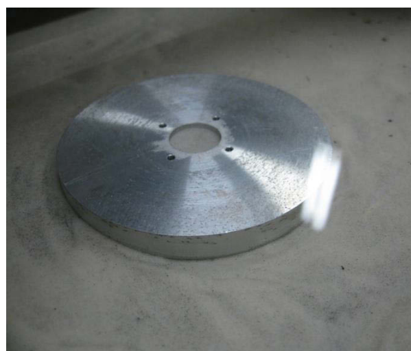
Figure 4-28. The rotated footing after test number four was completed (after Harloe 2010)
