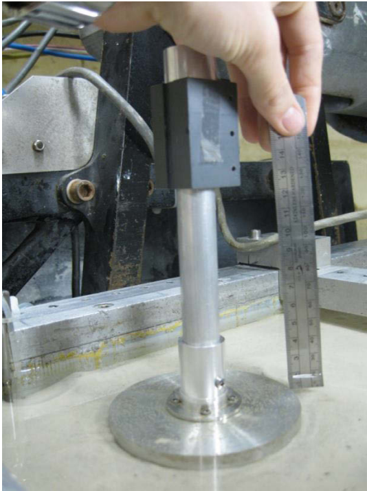
Figure 4-39. The water level was at the level of the bearing plate during the tests (after Harloe 2010)
