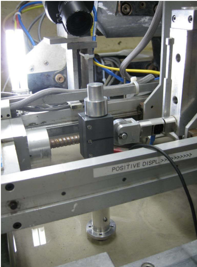
Figure 4-37. Test number eight (Single pile) installed in the centrifuge strongbox (after Harloe 2010)
