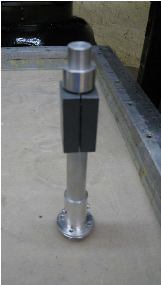
Figure 4-37. Test number eight (Single pile) installed in the centrifuge strongbox (after Harloe 2010)
