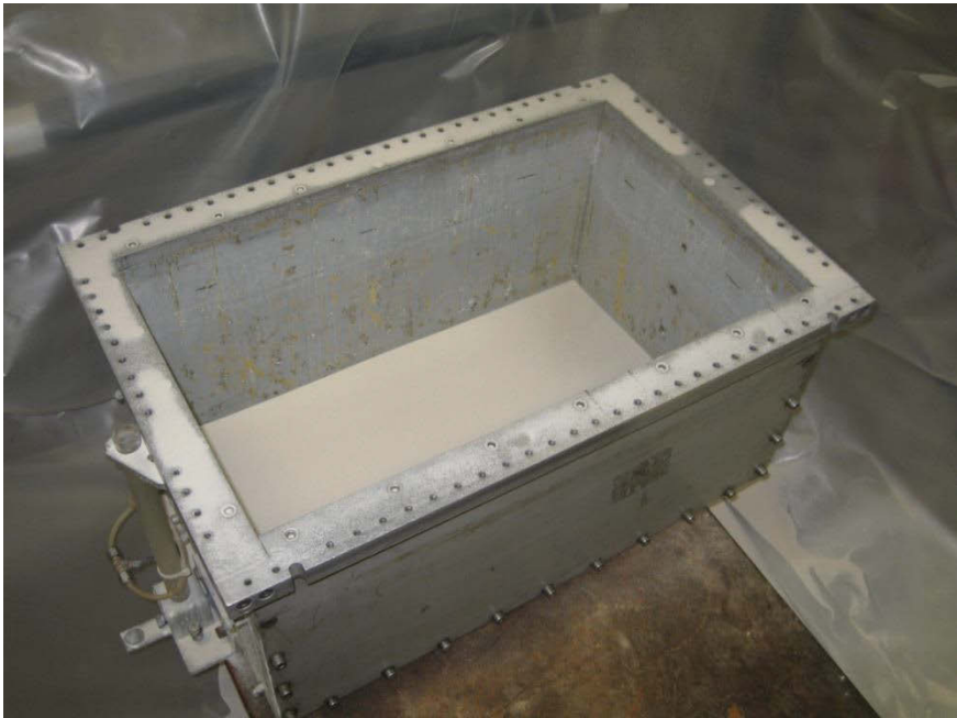
Figure 4-2. The strongbox used on the beam centrifuge (after Harloe 2010)
