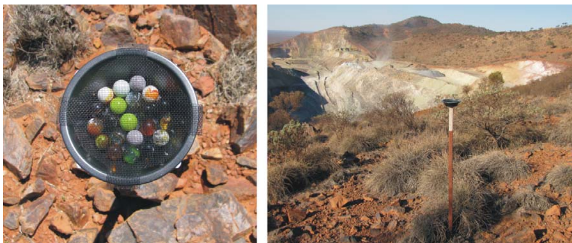
Figure 3: Dust collectors established at the Jack Hills. Left: topside view of dust trap; right: dust trap on stake adjacent to the mine pit, looking in a northeasterly direction.
