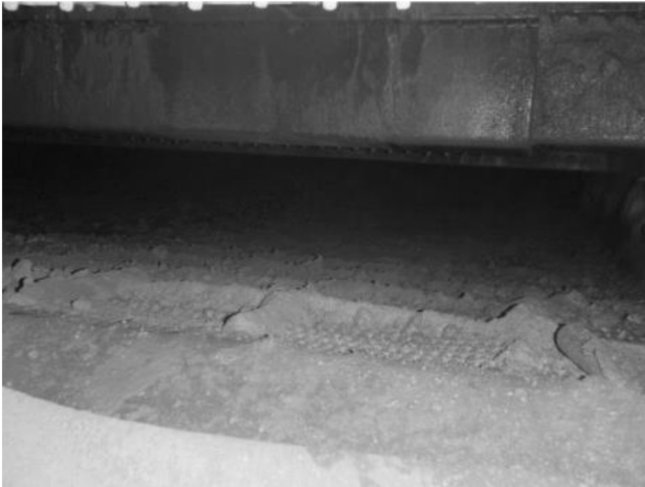
Figure 1: Accurate modeling of ochreous goethite is necessary to prevent handling problems such as this blocked screen. From Paine et al. (2016).
