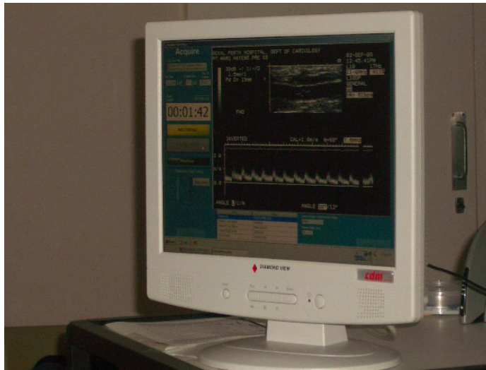
Figure 3-11: The computer used to image the blood vessel diameter and blood flow.
