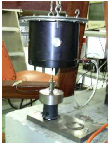
Figure 8.8. Graphic illustration of the experimental setup for shaker excitation of the rubber-mass system.
