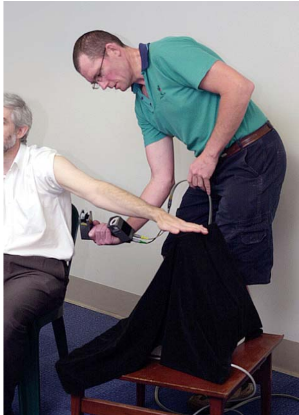
Figure IV.1: Demonstrates the use and orientation of FastSCAN scanning hand piece, including camera, while subject is positioned for 3D access of upper limb. (The transmitter is mounted beneath the black velvet cover.)
