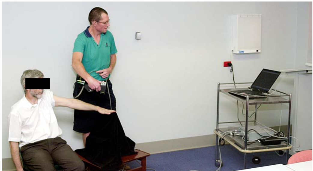
Figure 3.6: The candidate performing 3D laser scanning of a healthy subject upper limb
