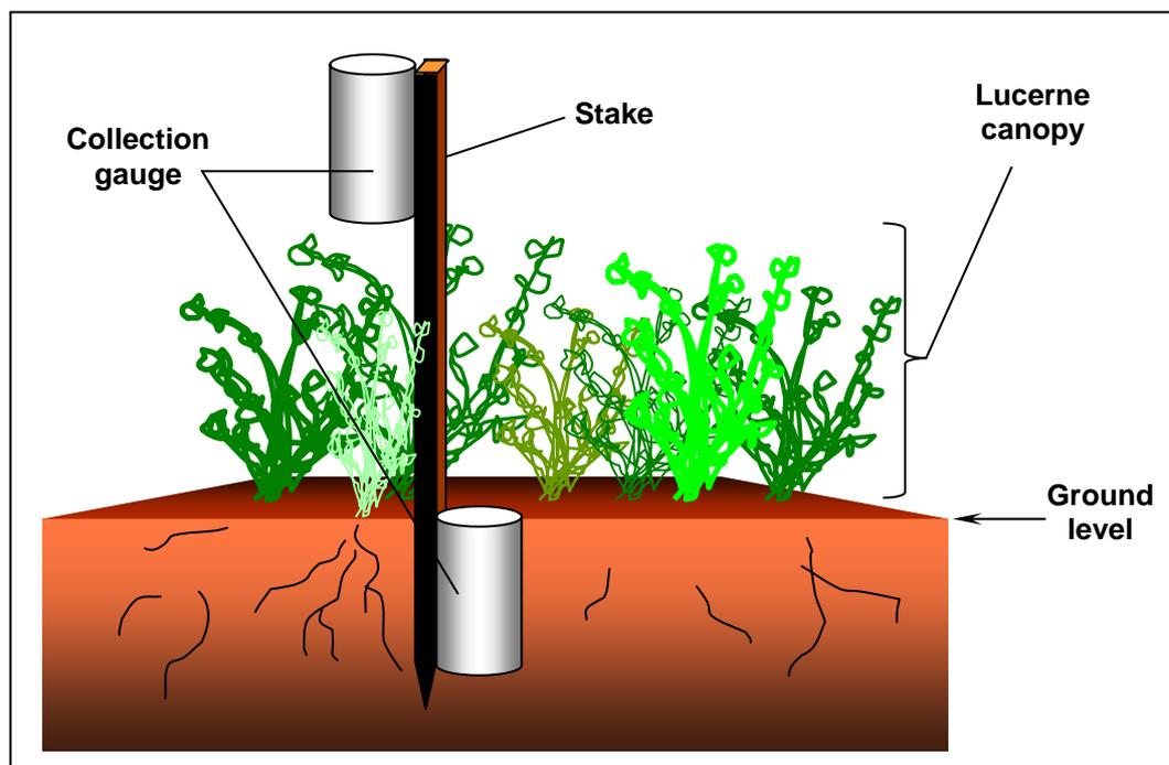
**Figure 7.6.** Configuration of vessels to measure interception of irrigation water by lucerne foliage.
