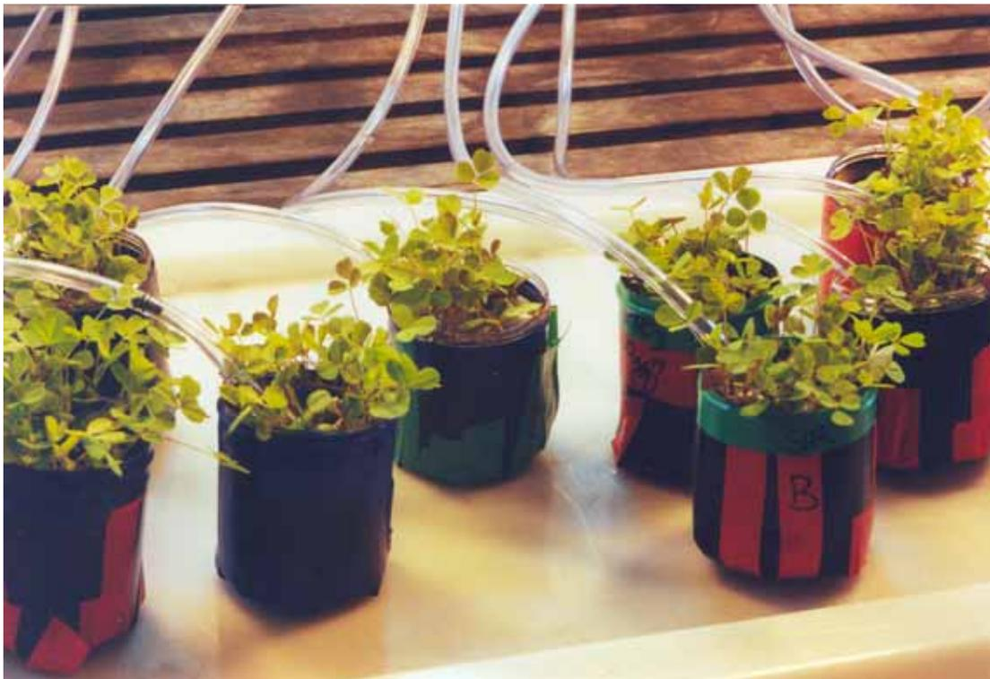
**Plate 6.2.** Equipment for root exudate collection (14 d). Vessels were covered in black plastic to minimise light on roots. Aeration hoses are visible.
