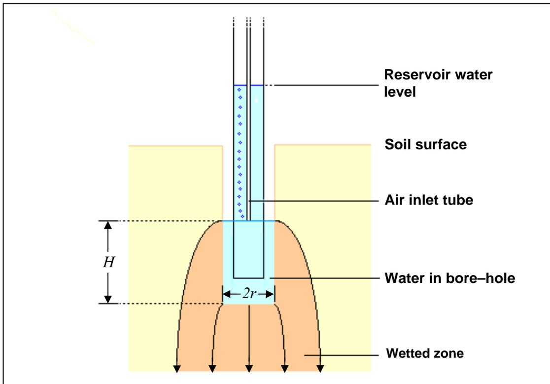
**Figure 7.3. The bore-hole permeameter for measuring sub-surface saturated hydraulic conductivity above a water table.**
