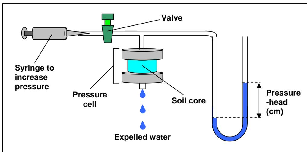
**Figure 7.4. Tempe® pressure cell arrangement to measure water retention from saturation to 100 cm soil-water pressure.**
