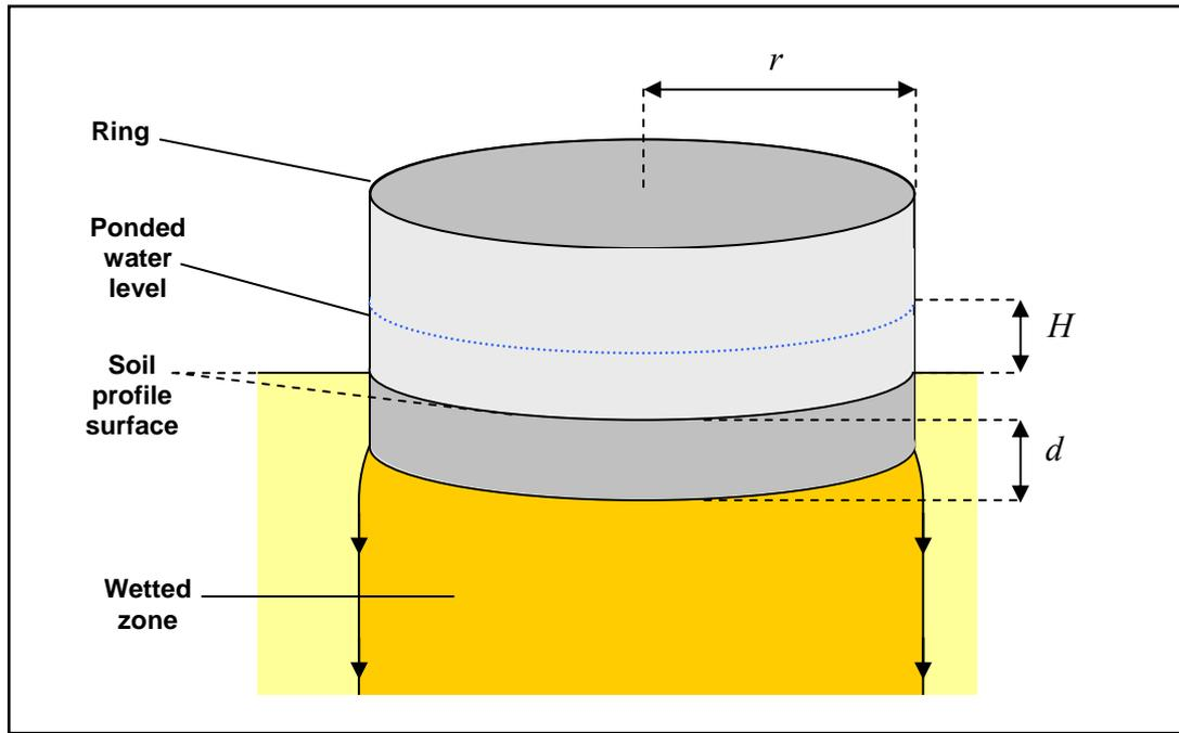
**Figure 7.2.** The ponded ring infiltrometer for “near-surface” measurement of infiltration and hydraulic conductivity.
