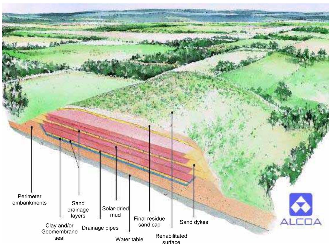
**Figure 1.1. Intermittent layers of bauxite residue sand and red mud through dry stacking in a residue disposal area leave a layer of residue sand as a final surface for revegetation (Alcoa World Alumina Australia, Environmental Department).**
