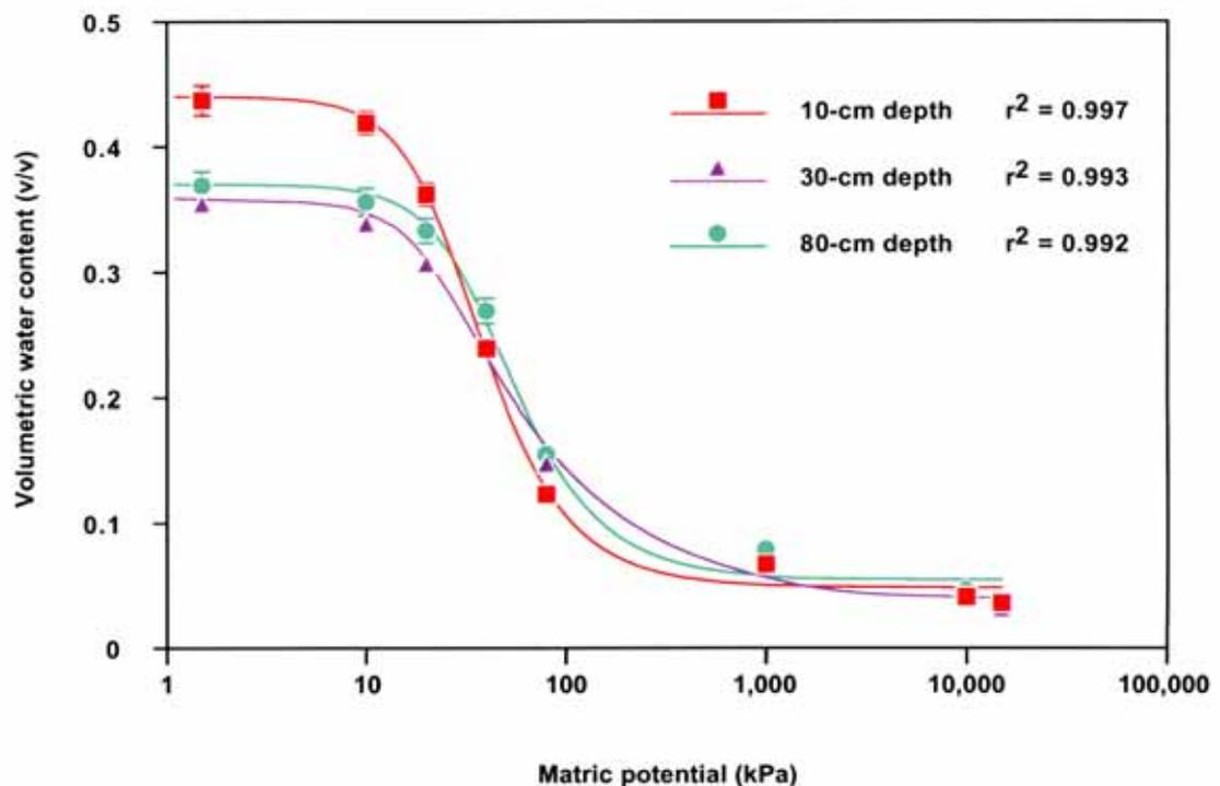
**Figure 7.7.** Observed water retention data and fitted water retention curves for bauxite residue sand sampled from different profile depths. Water retention curve parameters are given in Table 7.5.
