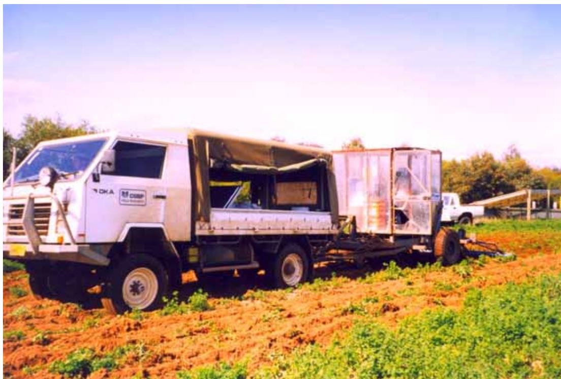
*Plate 5.1. Deep banding of manganese in lucerne pasture at the Pinjarra revegetated bauxite residue site*
