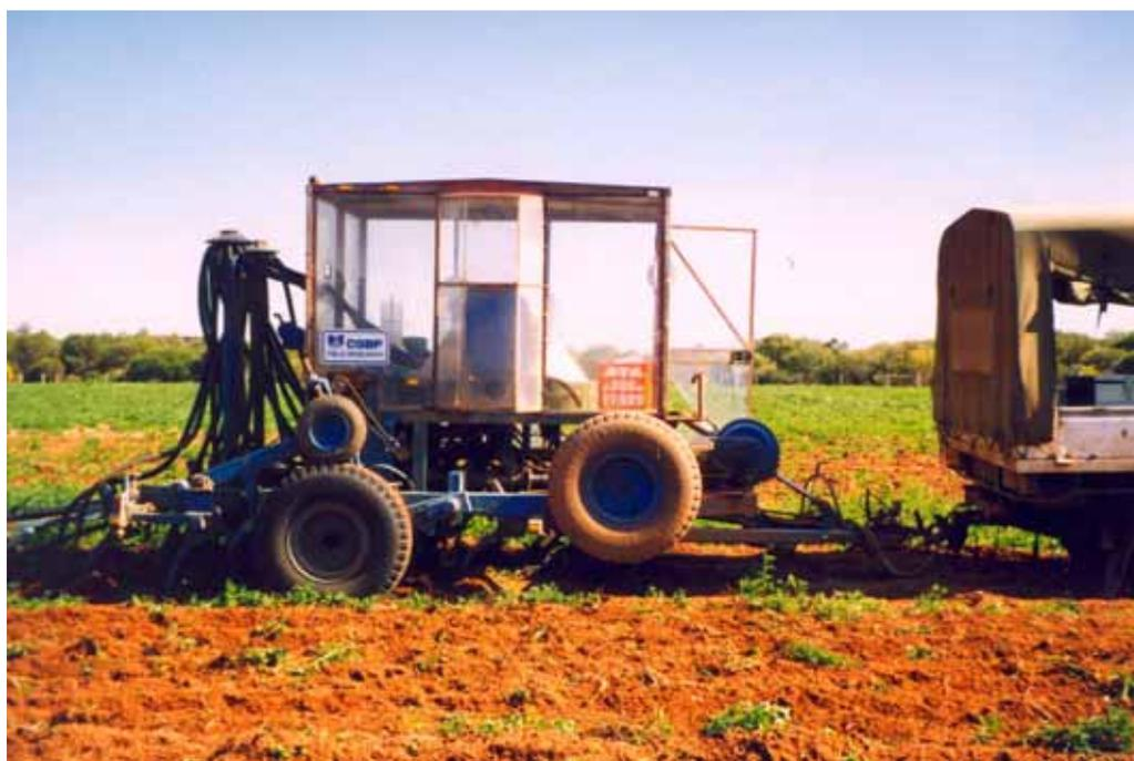
**Plate 5.2.** Equipment used for deep banding of Mn fertiliser at the Pinjarra site.
