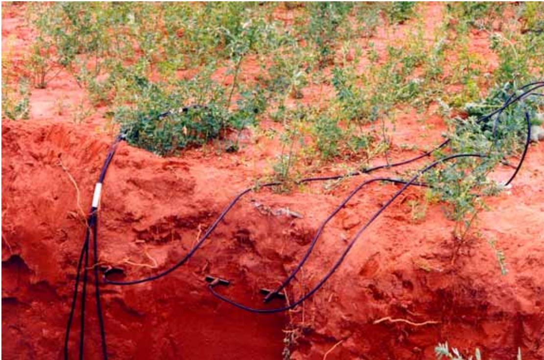
**Plate 7.3.** Buriable TDR probes inserted in triplicate at each depth (30-cm depth shown). Note prevalence of pale green, Mn-deficient lucerne foliage.
