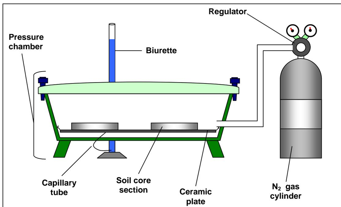
**Figure 7.5.** Arrangement of soil core sections in high pressure chambers.
