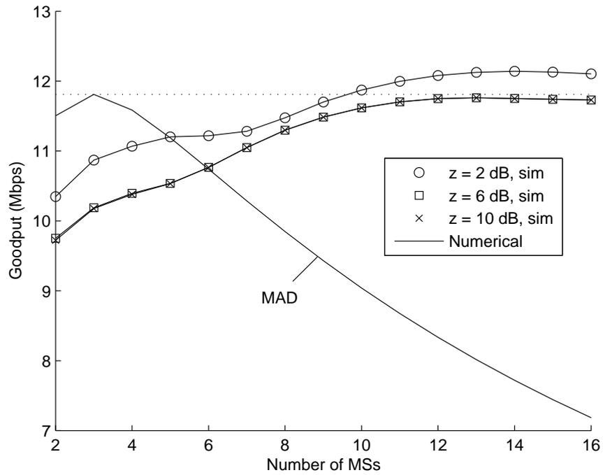
Figure 3.1: Expected goodput for MDC over Rayleigh fading channels at an average SNR of 17 dB.
