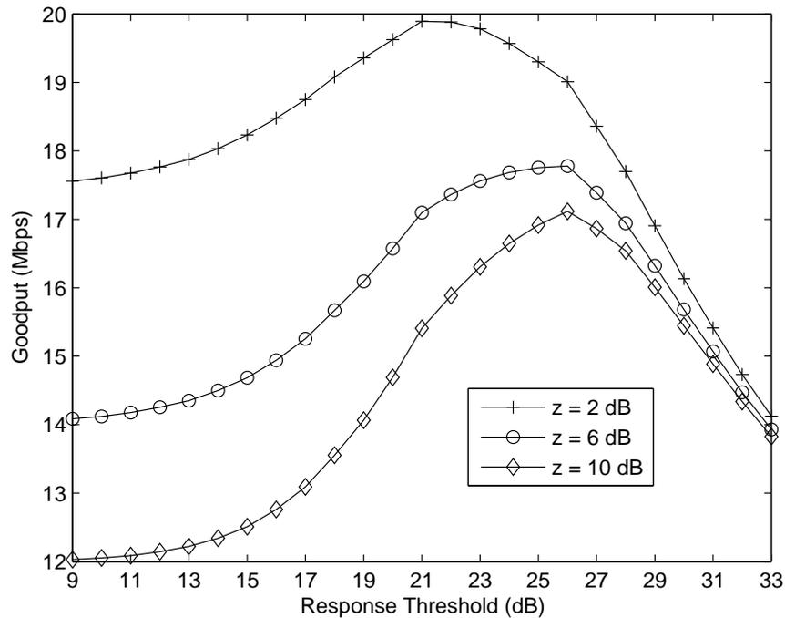
Figure 2.4: MDC goodput performance versus  $\gamma$  in a network with 8 MSs
