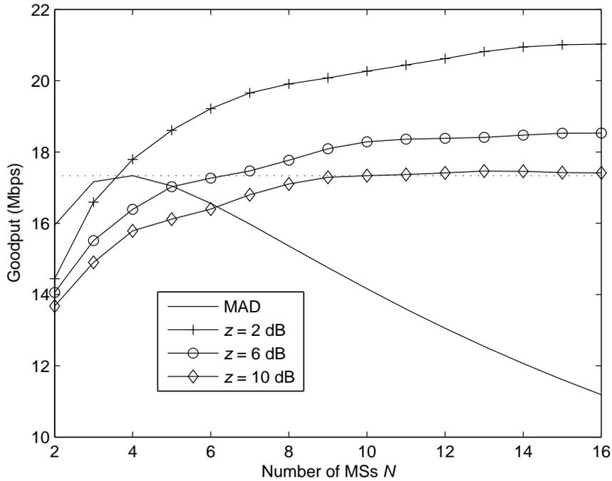
Figure 2.5: MAD goodput performance and MDC goodput performance with optimal response thresholds
