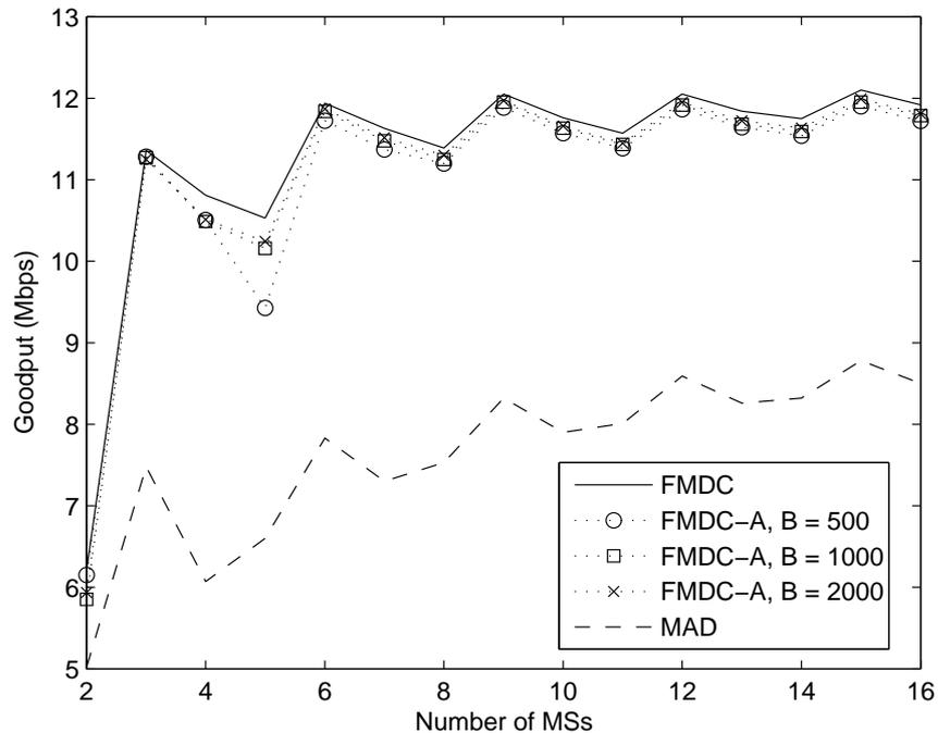
Figure 5.2: Goodput performance of FMDC-A over Type II channels with  $z = 2$  dB and step size  $s = 0.1$  dB.
