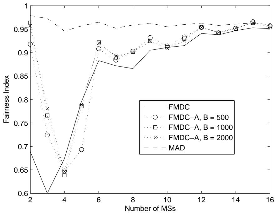
Figure 5.3: Fairness performance of FMDC-A over Type II channels with  $z = 2$  dB and step size  $s = 0.1$  dB.
