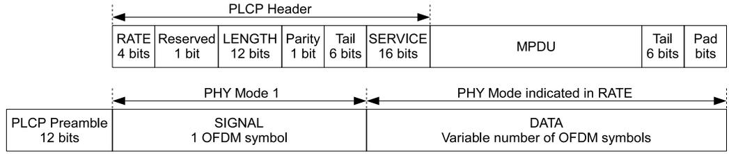
Figure 2.2: IEEE 802.11a PPDU frame format.
