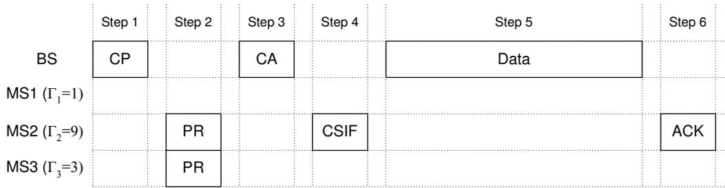
Figure 2.1: Example MDC transmission cycle for  $\gamma = 2$  and  $z = 2.5$ .
