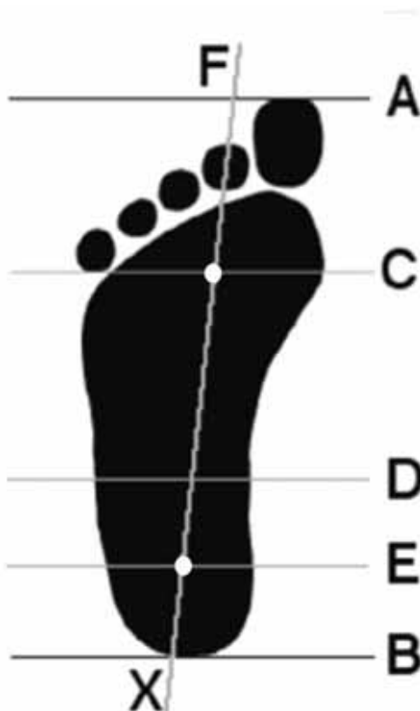
Figure 3.2: The length of the footprint was measured from (A) to (B) and divided into thirds (C) and (D), and the proximal third further divided into half (E). The width of the footprint was measured at 17% (E) and 66% (C) of the foot length and midpoints obtained giving the foot axis (FX) (adapted from Taranto et al) 6
