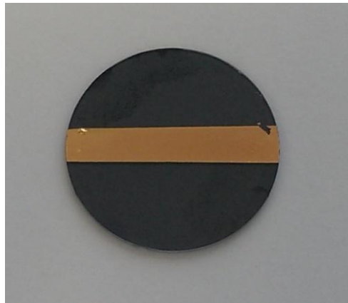
Fig. 4.1.5: Gold strip deposited across the middle of the QC845 coated quartz sample.
