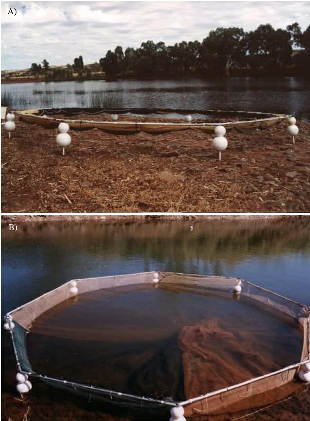
Plate 3.1. The drop-net. (A) the net gathered ready to be triggered, (B) the net after it has been triggered, gathered and brought to shore for dip net collection of the fish.
