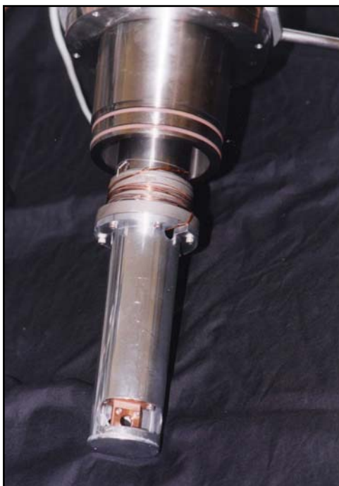
Figure 2.2: Radiation shield, cold finger and sample window
