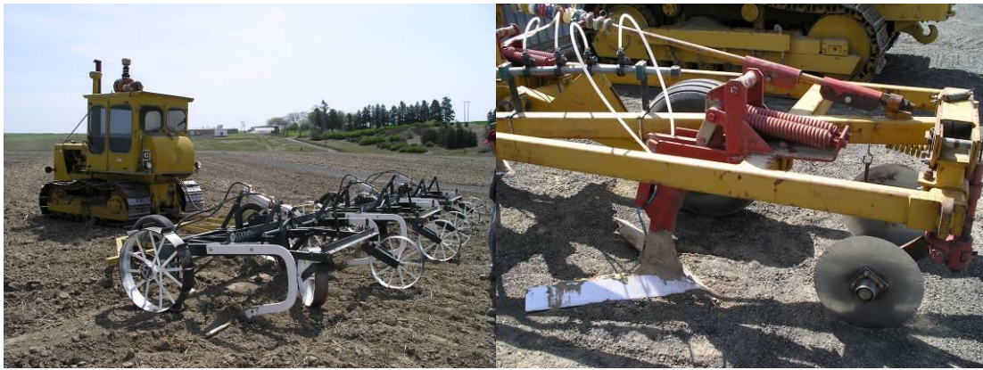
Figure 2.6: A rod weeder (left) and blade-cutter (right) in Washington State, USA. The rod or blades are pulled through the soil, below the soil surface, to cut plants free from their roots.
