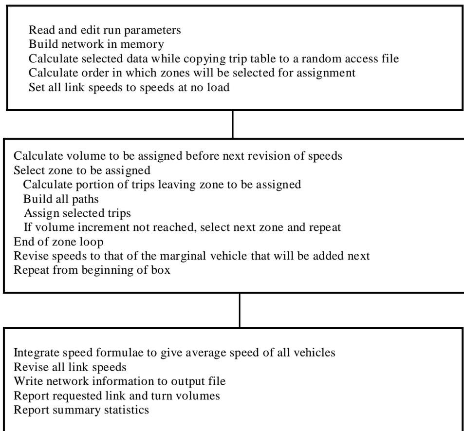
To achieve the effect of a reasonably continuous process, ie a small increment of trips on each link between capacity restraints, the total number of trips to be assigned needs to be broken into at least fifty steps. If this were done by taking the same percentage from all zones before revising the travel times, the amount of computer time would be excessive. The number of trips leaving a zone is not uniform over a whole network and
