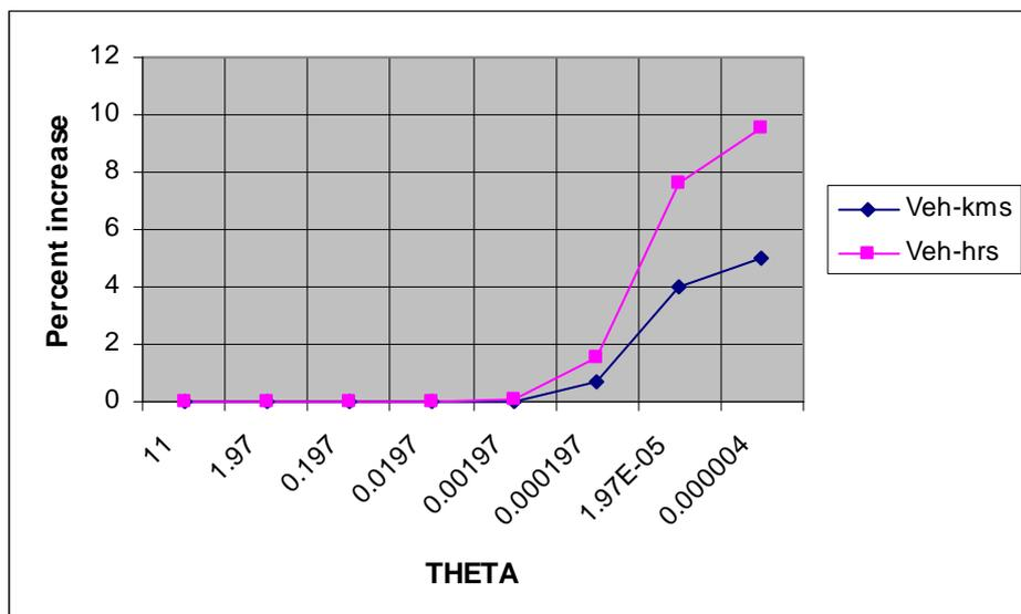
Figure 3.12 shows how lowering the value of  $\theta$  allows the sharing of traffic to paths with a bigger difference in length from the minimum path. This shows the desirability of using as low a value of  $\theta$  as possible consistent with not having traffic use unacceptable paths and acceptable paths being rejected when a new node number is added.
