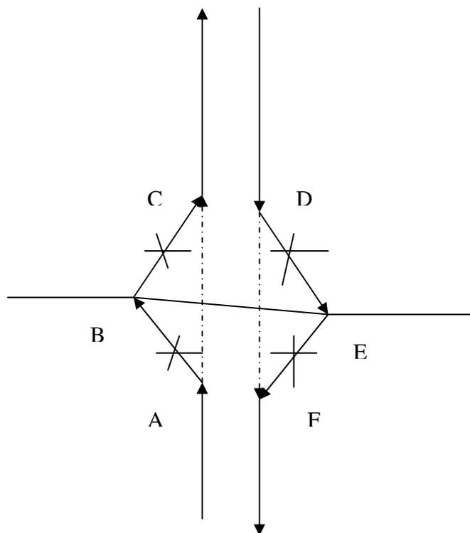
There is a second undesirable feature of Dial's multi path algorithm. This is described with reference to Figure 2.6. In Figure 2.6, both paths are possible when travelling from A to C and from C to A as in each case the terminating node (C or A) is further from the origin than the intermediate nodes B and D. If one were now to split the link AD in half by adding a node (E) in the middle, both paths from A to C are still possible. However,
