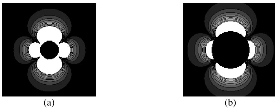
Figure 6-4 – Contour plot of the field gradients for a cylinder aligned orthogonal to the field.
