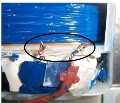
Figure 4.6-1 The Shorted Fuse
