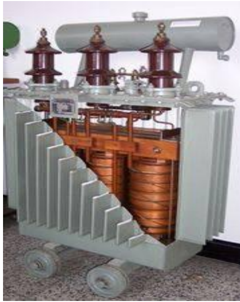
Figure 2.1-2 Oil Immersed Power Transformer
