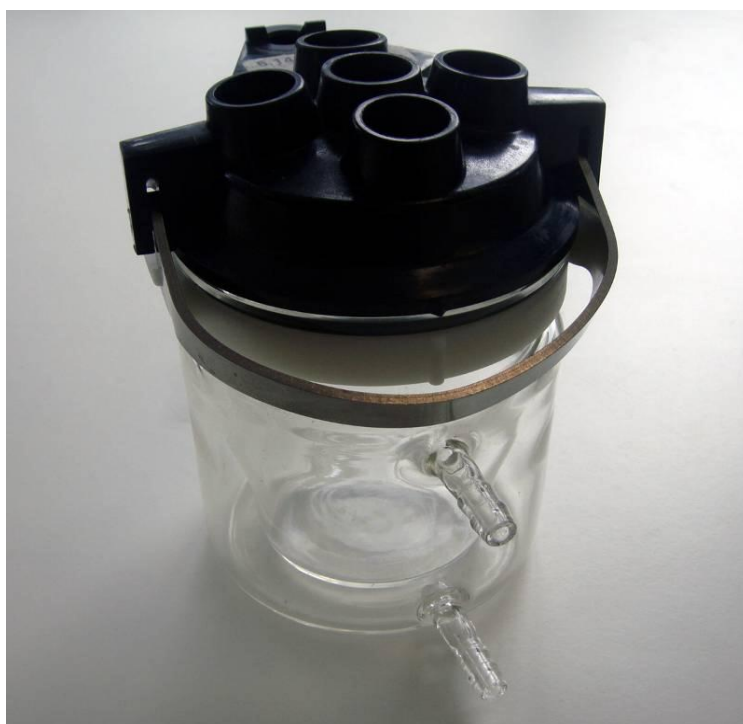
Figure 3-3 The three-electrode electrochemical cell with the lid
