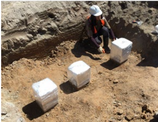
Figure 9. Excavated block samples, ready for preparation for transport.
