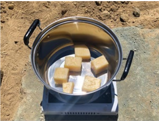
Figure 5. A small portable burner stove was used to melt wax blocks for sample preparation.
