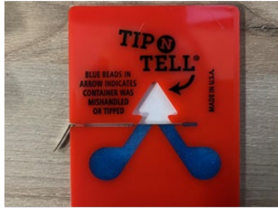
Figure 14. Tilt'n'tell indicators were affixed to each wooden box and pallet.
