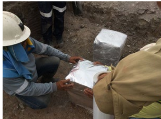
Figure 8. The wax-sealed and plastic-wrapped blocks were wrapped with aluminium foil and again with an additional layer of plastic wrap.
