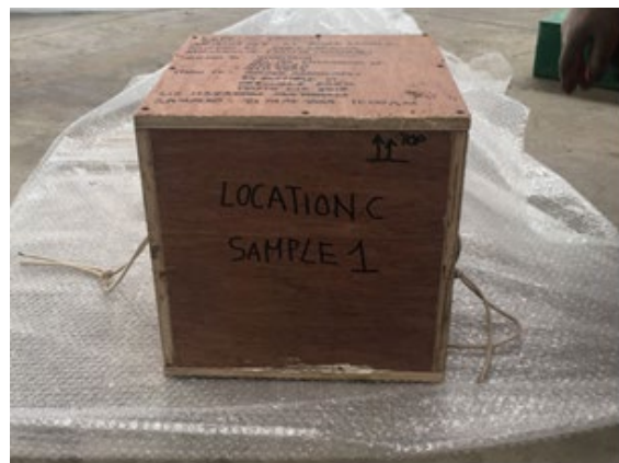
Figure 12. Lids were applied to the top and base of the wooden box when all voids were filled with eco foam.
