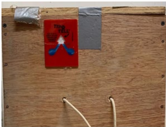
Figure 15. The tip'n'tell indicators sighted on arrival confirming the shipment had not tilted or tipped.
