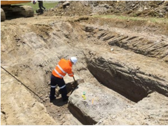
Figure 3. Excavation of the block samples through the use of hand tools.
