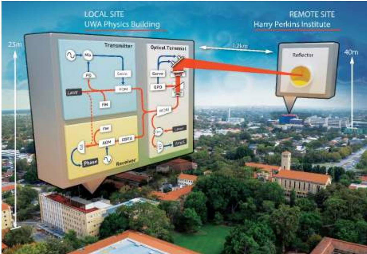
**FIG. 1.** Simplified schematic of the phase stabilization system integrated with the optical terminal. Blue lines, RF signals; and red lines, optical signals. AOM, acousto-optic modulator; Circ., circulator; FM, Faraday mirror; Mix, RF mixer; PD, photodetector; QPD, quadrant photodetector; EDFA, erbium-doped fiber amplifier; and WDM, wavelength-division multiplexer.
