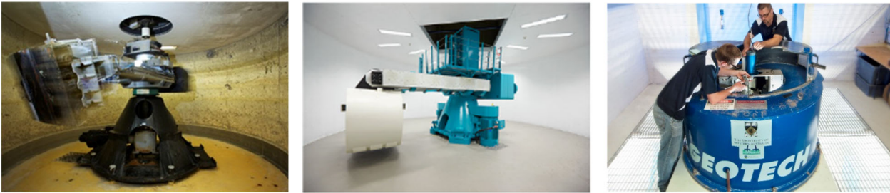
Figure 4 The NGCF centrifuges: 3.6 m diameter beam centrifuge (left), 10.0 m diameter beam centrifuge (middle) and 1.2 m diameter drum centrifuge (right)
