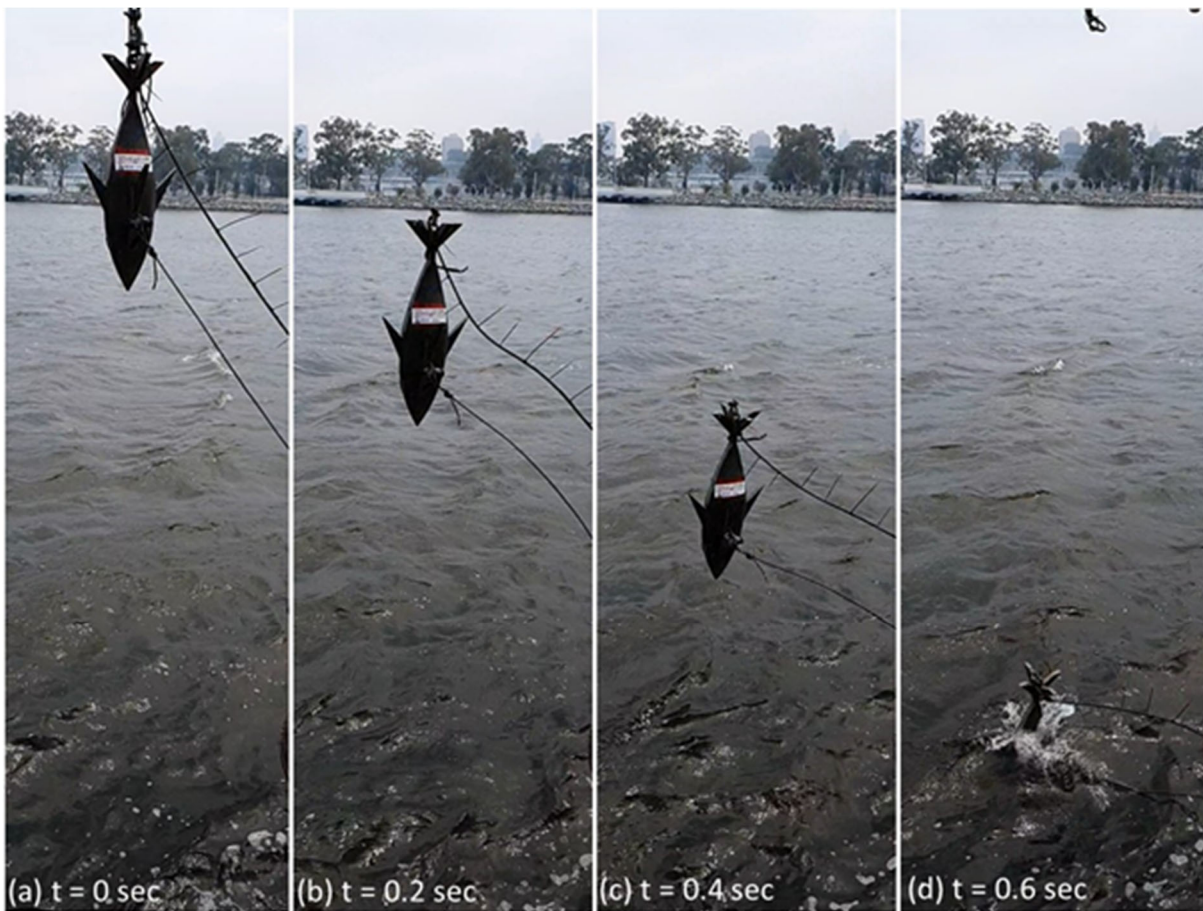
Figure 10 Prototype trials of the ‘fish’ anchor in the Swan River, WA
