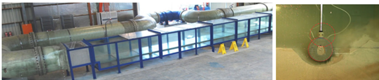
Figure 6 Large O-Tube facility. Right, scour around a model pipeline – current from left (Draper et al., 2015)
