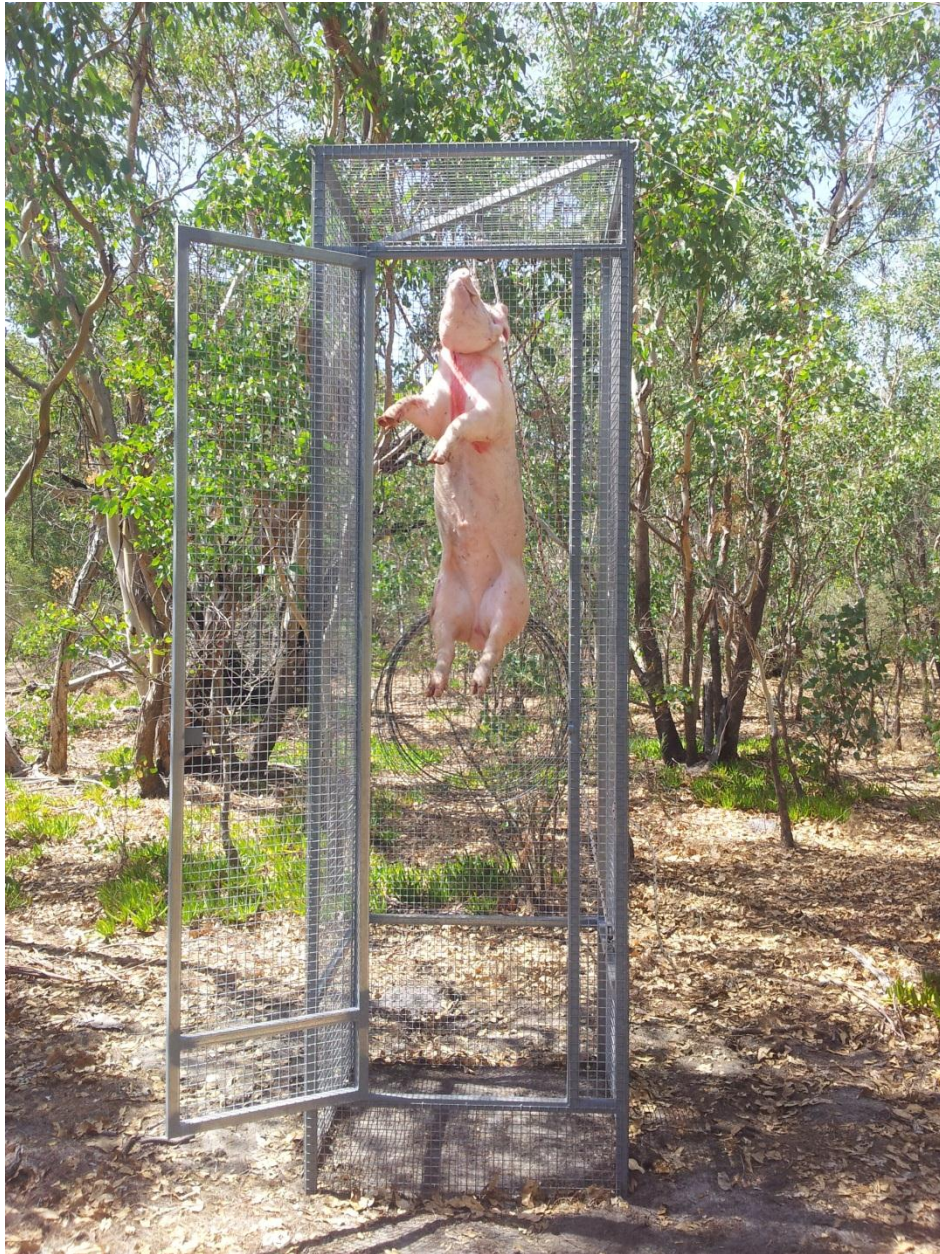
Figure 2. A representative example of the steel cage use to protect hanging carcasses from animal predation during the trial periods. The cage had a swing door which acted as an entry point for sampling throughout the trial.,
