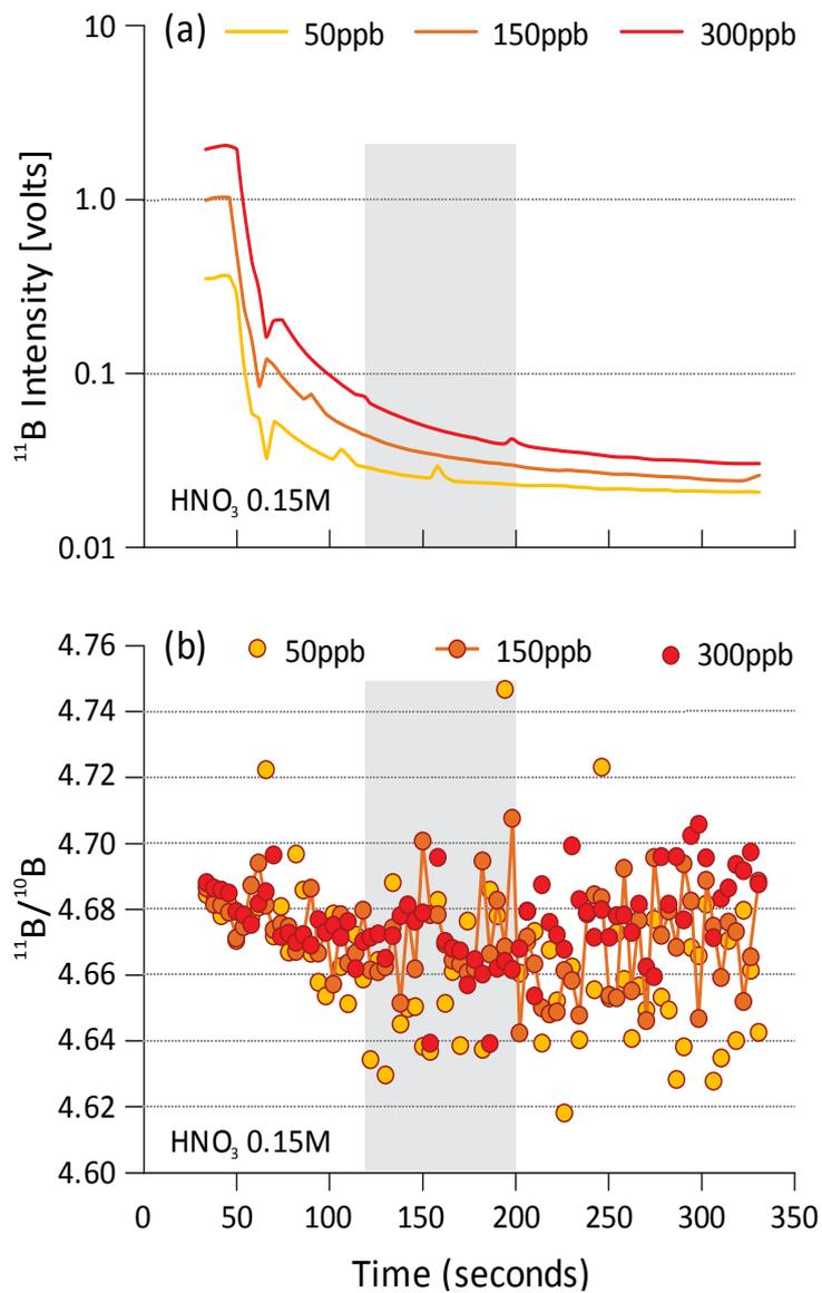
**Figure 2.** (a) Boron washout with 0.15N HNO<sub>3</sub> following introduction of 50 ppb, 150 ppb and 300 ppb B solutions into a cyclonic quartz spray chamber (b) The  $^{11}\text{B}/^{10}\text{B}$  isotopic composition is shown as a function of washout duration after the measurement of the laboratory standard UWA24.7. The blank composition is measured during the interval from 120-200 seconds (shaded) and is relatively constant.
