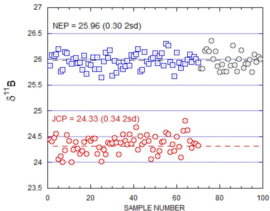
**Figure 5.** Plot of long-term variation  $\delta^{11}\text{B}$  compositions measured for the coral carbonate standards JcP-1 ( $\delta^{11}\text{B} = 24.33 \pm 0.34\%$  2sd) and NEP ( $\delta^{11}\text{B} = 25.96 \pm 0.30\%$  2sd). For NEP the open circles are from measurements using the NEPTUNE Plus while blue squares are from measurements using the NU Plasma II, with both giving identical results. The JcP-1 standard was measured using the NU Plasma II.
